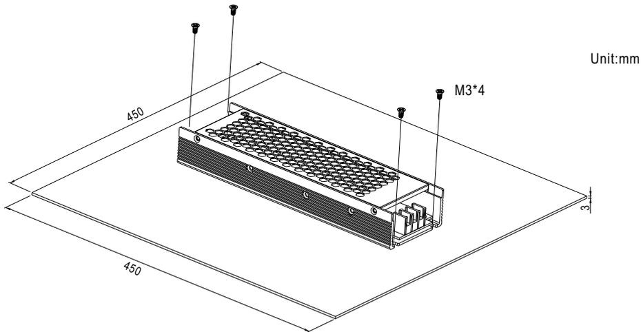
2. For heat dissipation, at least 5cm installation distance around the PSU should be kept, shown as below:
