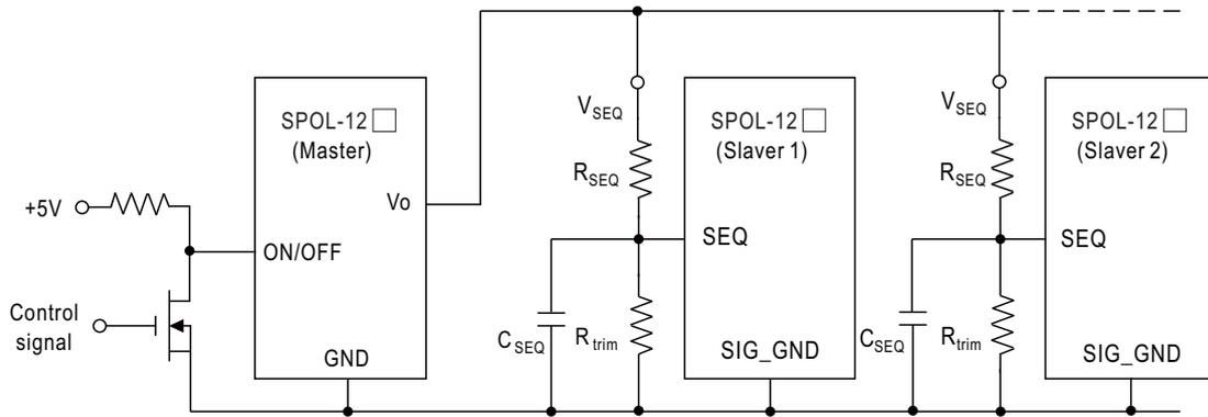
Schematic for Output Sequencing
