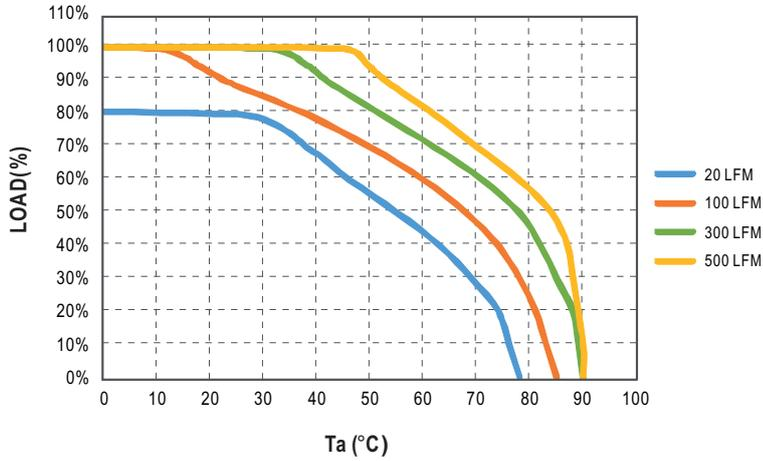
The derating curve was measured at 12V input and 5V output., all of the element can't be higher than 125°C.
