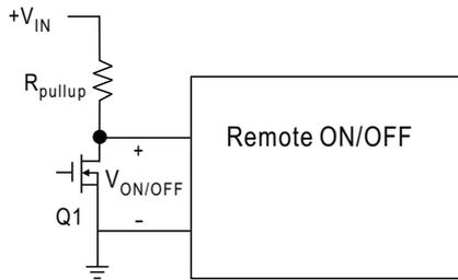
The circuit configuration for using the Remote ON/OFF pin is shown in figure. And the logic type active mode as the description below.
